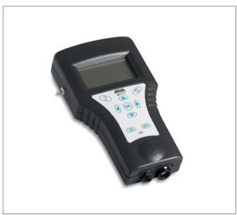
For pin-pointing of cable faults the digital Universal Locator UL 30 is used with ground microphone BM 30 and Surge Voltage Generator (SSG/STG). With its integrated acoustic propagation time measurement the UL 30 displays the distance to fault in meter and indicates the position if the the fault is reached. The special feature of UL 30 is the calculation of the fault distance between two manholes.
