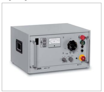
The Surge Voltage Generators are used for pre-locating as well as for pin-pointing of high and low resistance faults in power cables. The stored energy of the high voltage capacitors is fed at intervals in to the faulty cable. This causes an acoustic noise at the fault position which can be detected with a ground microphone and an audio frequency receiver.
