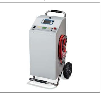
The SYSCOMPACT 2000 M is a mobile and multifunctional cable location system. The surge and test generator is designed for the testing of cables and sheaths and for the precise location of high-resistance and intermittent faults.
