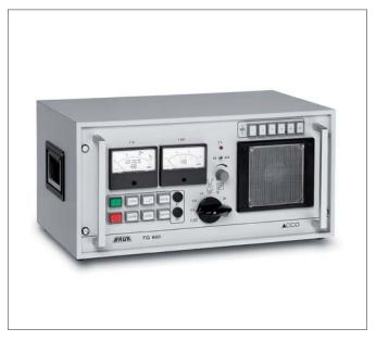
The high performance Audio Frequency Transmitter TG 600 is especially designed for accurate location of cable faults and joints according to the twist method. The display of input and output current enables optimised impedance matching.
