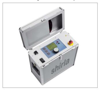
The fault location system is used for cable- and cable sheath testing, fault prelocation as well as for sheath fault pinpointing according to Murray and Glaser.
