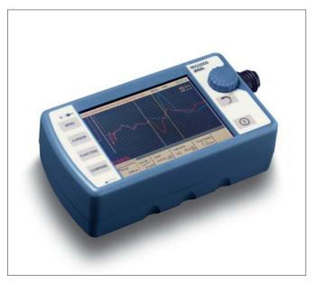
The Pulse Reflection Test Set IRG 2000 is a portable, easy to use, single-phase unit for cable fault pre-location using the Time Domain Reflection (TDR) method on low, medium and high voltage cables. It can also be used on live cables up to 400 V. Further fault location methods are available with the application of the appropriate coupling device. Its measuring ranges enable pre-location on cable lengths from 0 m to 65 km (0 to 213,000 feet).
