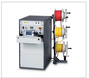
The SYSCOMPACT 1000 is a multifunctional cable fault location system for use in low-voltage networks. The STG Surge and Test Generator are designed for testing of cables and cable sheaths and for precise location of the high-resistance and intermittent faults.
