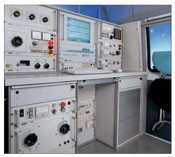
Modified to suit your requirements and vehicles, BAUR offers you a number of systems in various ergonomic designs for individual device installation. We have drawn on years of experience to develop tried and tested standard systems. Four standard systems for pre-location and pin-pointing of cable faults, testing and diagnosis are combined to suit your application.
