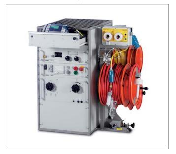
The SYSCOMPACT 2000 is a multi-functional cable fault location system in a modular 19" plug-in design. The surge and test generator is designed for testing of cables and cable sheaths and for the precise location of high-resistance and intermittent faults.
