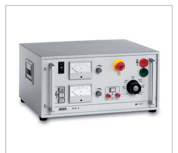
The burn down transformer ATG 2 enables the user to change a high resistance fault into a low resistance fault. Thus allowing an Impulse Reflection Test Set to be used for low resistance fault prelocation.
