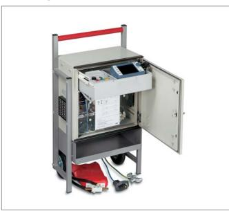
The Live Locator EF 24/200 is mainly used as an adjustable, fast electronic fuse in low voltage power cable distribution networks. In combination with the Pulse Reflection Test Set IRG 2000 it enables to locate high resistance and intermittent faults on live cables even with connected consumers. The Live Locator can be used as a surge switch and for pulsing of mainspower. This allows cable fault pin-pointing together with a ground microphone and audio frequency receiver.
